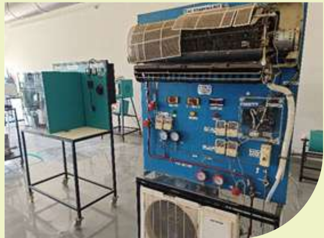
Split AC Test Rig
